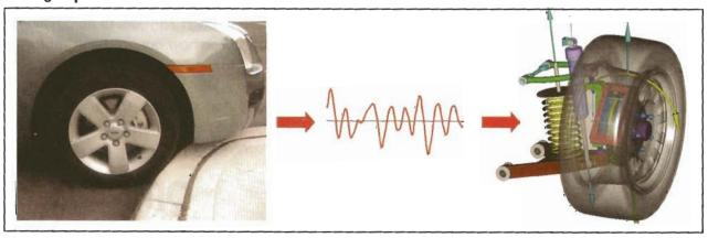
Data from test or analytical calculations can be used to define mechanism motion. Here, motion of the control arm is recorded as a function of time as a car drives over a curb. The test data are used to move the suspension assembly model in motion simulation.
