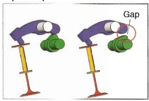
Impact and contact can be simulated, for example, to study a gap that may form between a cam and follower (rocker) in a valve lifting mechanism.
