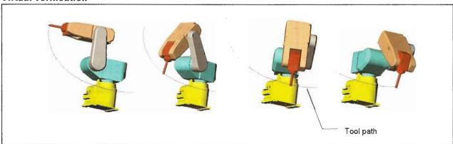
Simulated movement of an industrial robot through several positions makes it possible to create a tool path without physical tests.
