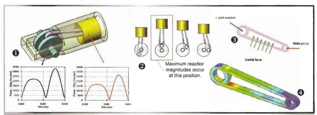
• Motion simulation finds reactions on both ends of the connecting rod: the large diameter end, which is the crank throw end, is attached to the crank shaft, and the small diameter end or wrist pin end, is attached to the piston by a wrist pin. Simulation also finds inertial forces acting on the connecting rod. These inertial forces are not negligible in fast-moving mechanisms. Plotted are reactions during one full turn.
